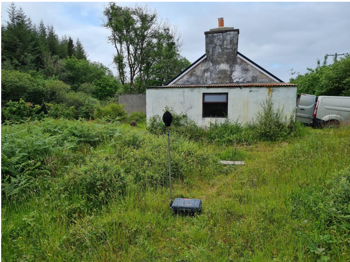
Figure 12-4: Noise Monitoring Installation – NML-2
